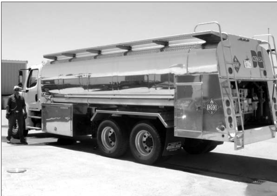
Aaron Brown with Sublette Co-op's new 2007 Freightliner 4500-gal fuel truck featuring five compartments, dual pumps, and semi-automatic transmission.
